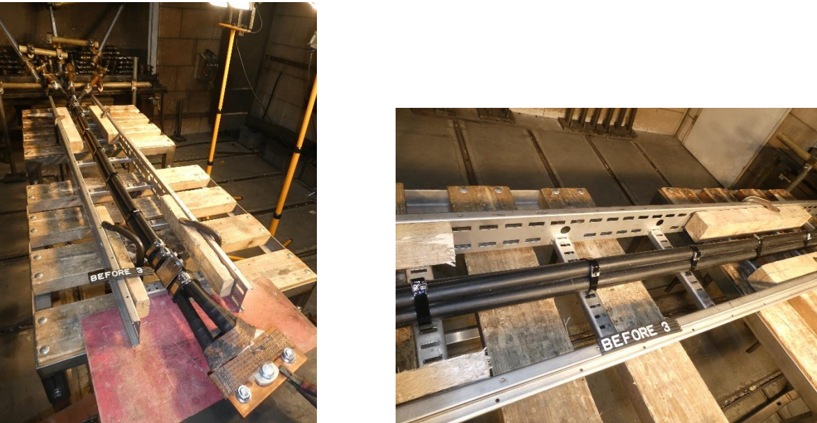
Photo 1 and 2 Cable cleats for electrical installations Manufacturer: Band-it IDEX Test rig number: 1
