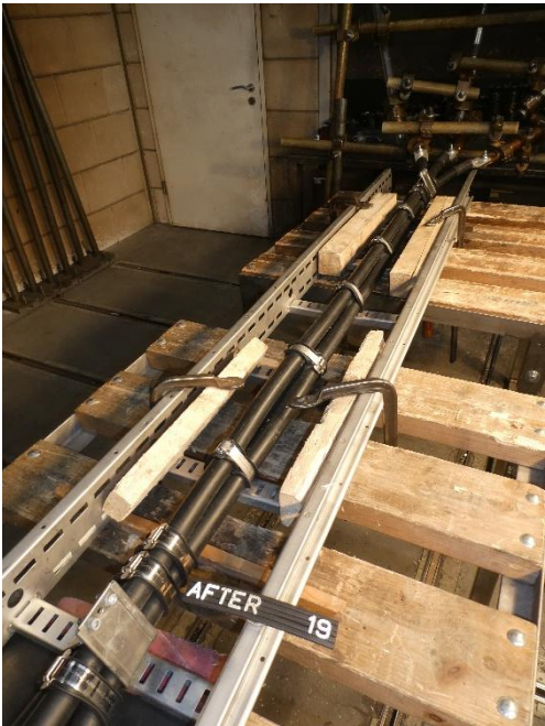
Photo 1 Cable cleats for electrical installations Manufacturer: Band-it IDEX Test rig number: 5
