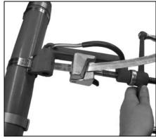
5. Roll tool over buckle, backing off with tension handle throughout entire rolling operation. Failure to back off with tension handle through-out entire course of rollover may result in breaking of band. There is no loss of tension as band released is used up in the bend.
