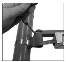
6. Pull cutting handle to cut the band. When applying ¾" Giant clamps, prior to cutting off clamp, release band gripper and push tool nose away from buckle approx. ¼".
