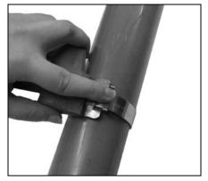
4. Place finger on BAND-IT Band at buckle bridge while tensioning with tool handle. When you feel BAND-IT Band stop moving through buckle as you are turning handle, maximum pressure is being exerted by the BAND-IT Band around object being clamped. Stop turning handle.
