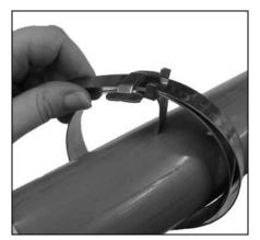
2. Continue band around object once more and again through buckle. Double banding develops a great deal more radial compression than single banding. Bend end of band under buckle.
