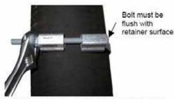
Insert the carriage bolt into the sliding retainer. Make sure the carriage bolt locks into place on the fixed retainer. Install a washer (not provided) if required. Install the nut and tighten until equipment is secure and all slack has been removed from band.
