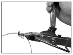
2. Form a clamp by threading the band through buckle and make a fold under the buckle. Insert tail of clamp into head of tool and slide into slot of winding mandrel. Depress locking pawl and tension clamp with forward strokes of the ratchet wrench.
