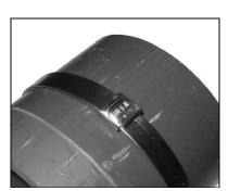
**9.** Complete clamp by tapping lip of band over buckle and remove ratchet wrench from tool as shown in step 6.
