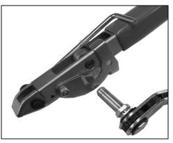
**6.** Remove band wrapped around winding mandrel by lifting up on locking pawl. Reverse ratchet and withdraw tensioning wrench from tool.
