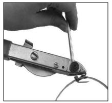
**4.** Cut off excess band by lifting cutter lever.
