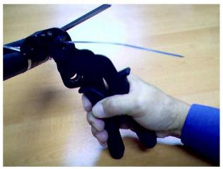
3. Squeeze tool repeatedly untill desired tension on the Ball-Lok Tie is reached.
