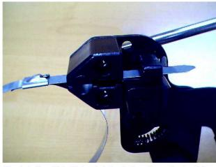
2. Slot tail of Ball-Lok Tie into the slot of the tool, push nose of tool against the buckle.
