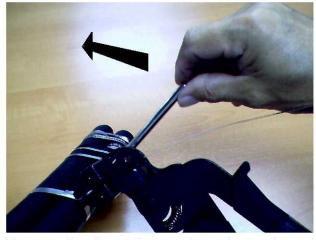
4. Turn cutter lever forward as shown to cut off excess tail end.
