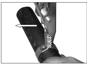
**4.** While holding tension with wrench, pivot tool up against buckle, then backward several times to break off clamp tail.
