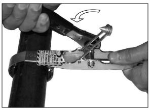
**2.** Start "pumping" ratchet wrench forward until proper tension has been applied.
