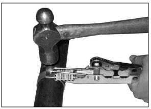
**3.** Place punch on clamp and while holding tension with ratchet wrench, lock clamp by striking punch once or more with hammer, depending on object being clamped.
