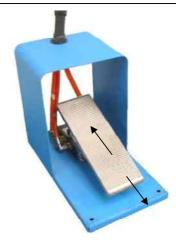
Dual function foot control valve. Pressing forward activates clamp installation. Heel action activates tail return and prepares for next clamp.
