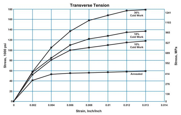
Like other austenitic stainless steels, type 201 does not exhibit a well defined transition from the elastic to the plastic range. For this reason, its yield strength is conventionally defined as the stress at which a line drawn with the initial slope of the stress-strain curve and the offset 0.2% on the abscissa intercepts the stress-strain curve.
