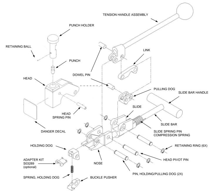
INSTRUCTIONS: DISSASSEMBLY AND ASSEMBLY OF PUNCH
