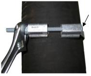
Bolt must be flush with retainer surface
