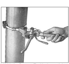
1. With the Bantam Tool in the straight or angle position, place the band in the nose of the tool and with sufficient band in the winding mandrel.
