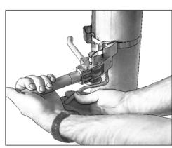
3. Roll tool over to the other side and pull the cutter handle. Remove tool and tap down ears of clip to complete clamp. Remove excess material from winding mandrel.
