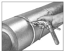
1. With the Bantam Tool in the pistol grip postion, place the band in the nose of the tool and with sufficient band in the winding mandrel.
