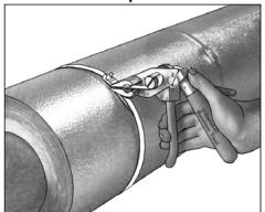
2. With ratcheting action, tension the band until clamp is tight. If necessary, band may be reposition by releasing tension with levers.
