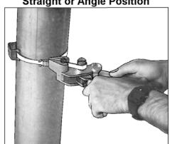
2. Move the ratchet handle back and forth until sufficient tension has been applied.
