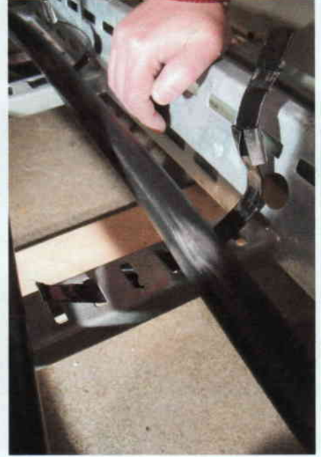
Close up of failed band.
