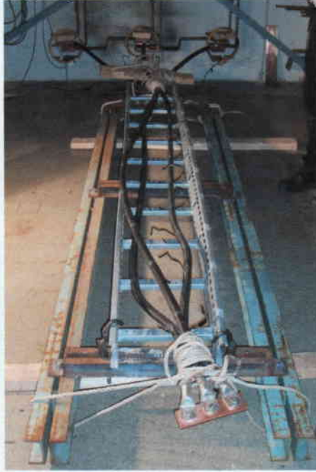
All bands failed on single wrap.
